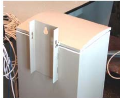
Figure 4: Sunshield installed on the top of the test sample
