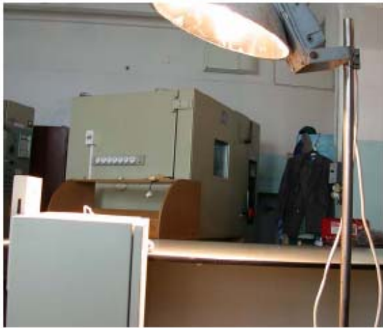
Figure 1: Exposure of the test sample to solar radiation simulator at 60° to the top surface
