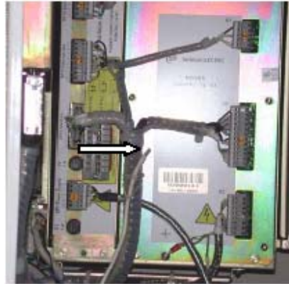
Figure 7: Location of middle temperature sensor inside of the test sample
