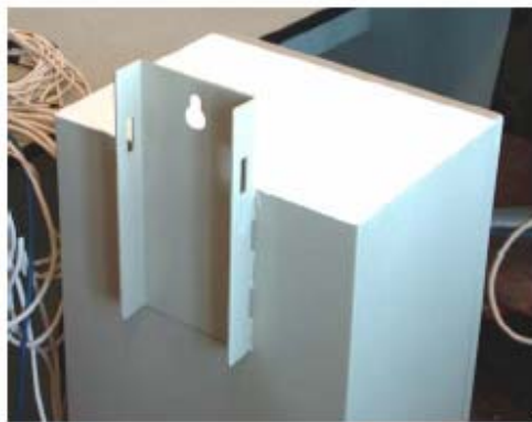
Figure 3: Thermal-Coat applied to the top surface of the test sample
