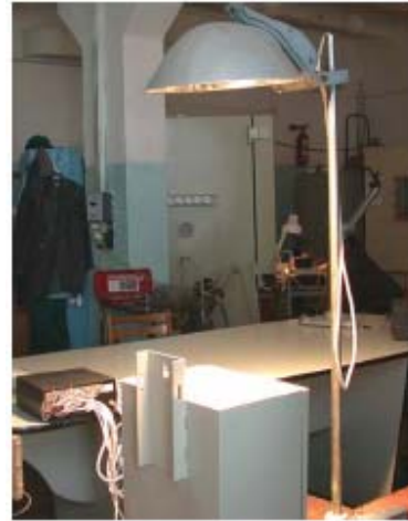
Figure 2: Exposure of the test sample to solar radiation simulator at 90° to the top surface
