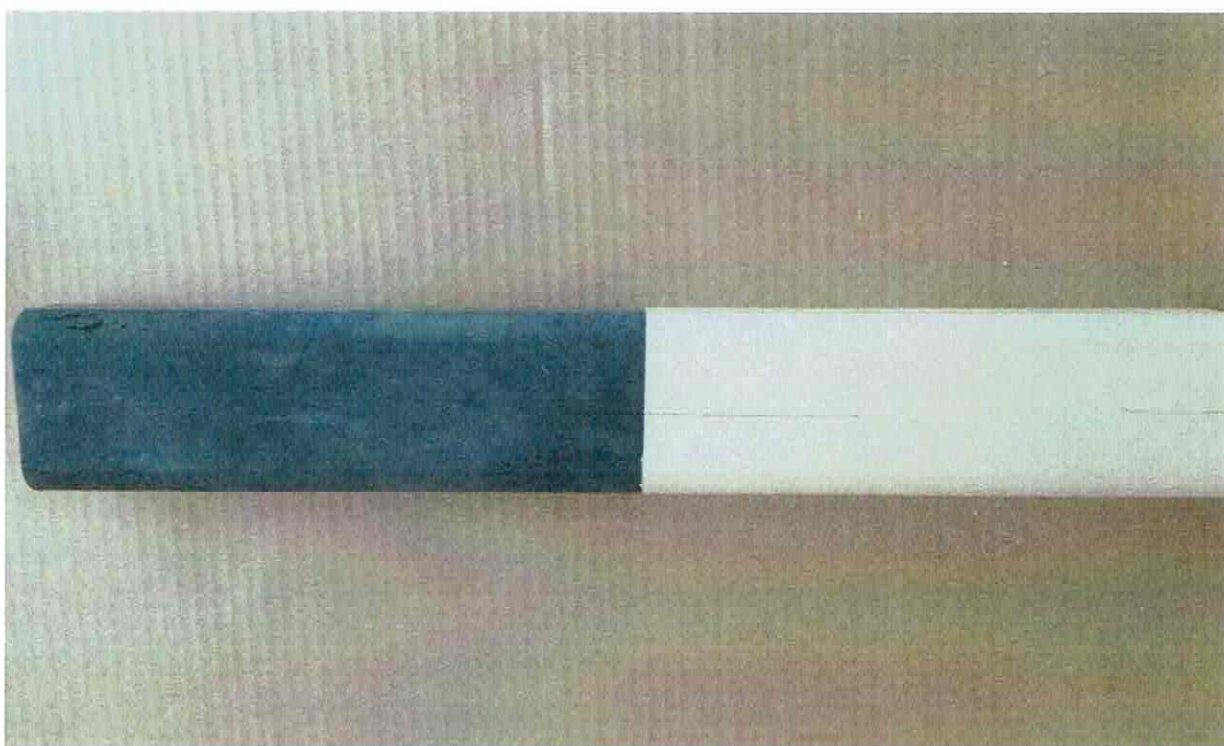
Photo 10. Condition after Two Exposure Cycles. MCU Paints. Test Piece #2.
